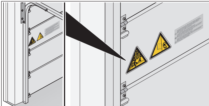
Fig. 1.2 Attach sticker on door panel
